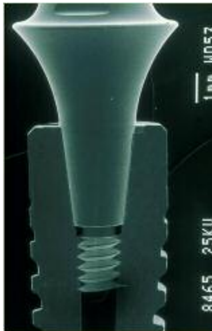
Fig. 10b: Morse taper invisible micro-gap.
